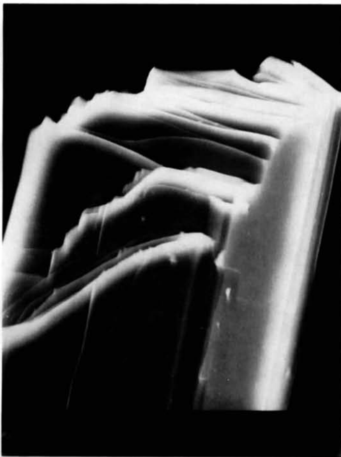
Fig. 3. Electron microscope photograph (magnification: 4500\times ) showing the cleavage planes in an \text{H}_2\text{Te}_2\text{O}_6 single crystal.
